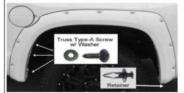
Apply 3 Truss Type-A screws with washers through 3 holes in the most front of the flare and into the factory holes on the wheel well. Install the retainer into the factory hole on the underside of the flare. Ensure the flare is on in the proper position, tighten all screws.
