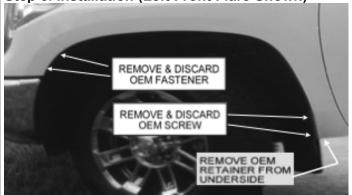
Remove 2 factory fasteners from front wheel well. Remove 2 factory screws from factory mud guard. Remove a push-in retainer from underside of the mud guard. Remove the factory mud guard.
