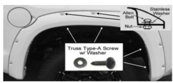
Use Hex Key to tighten the allen bolt & nylon nut firmly on every pocket of the fender flares. DO NOT OVER TIGHTEN! Hold the flare firmly and apply 2 Truss Type-A screws with washers through 2 holes in the tope of the flare and into the factory holes on the wheel well. Apply 2 Truss Type-A screws with washers through two holes in the most rear of the flare and into the factory holes on the wheel well.
