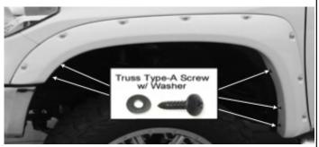
Apply 3 supplied Truss Type-A screws with washers through three holes in the rear of the flare and into the factory holes on the wheel well. Apply 2 Truss Type-A Screws with washers through two holes in the most of flare and into the factory holes on the wheel well. Ensure the flare is on in the proper postition and tighten all screws.
