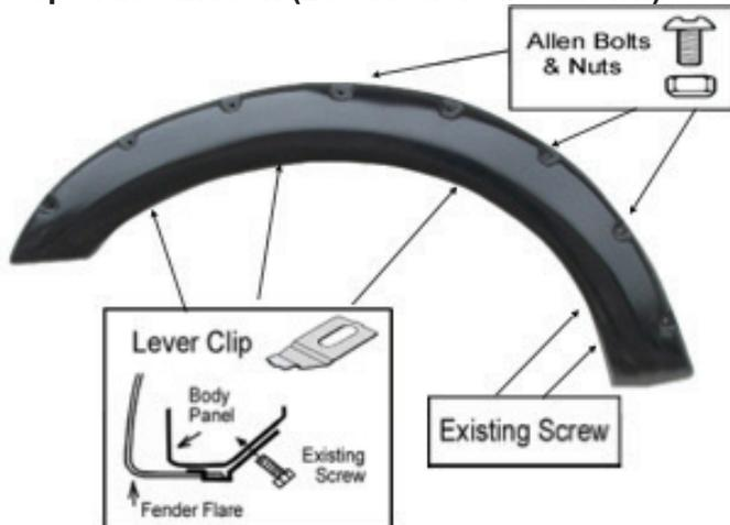
Use torx bit to tighten allen bolt & put firmly on every pocket of the fender flares first. Place the flare on the vehicle. Apply 3 Lever Clips secure it to the hole with existing screws as shown. Fasten the existing 2 factory screws into the original location that were preciously removed.
