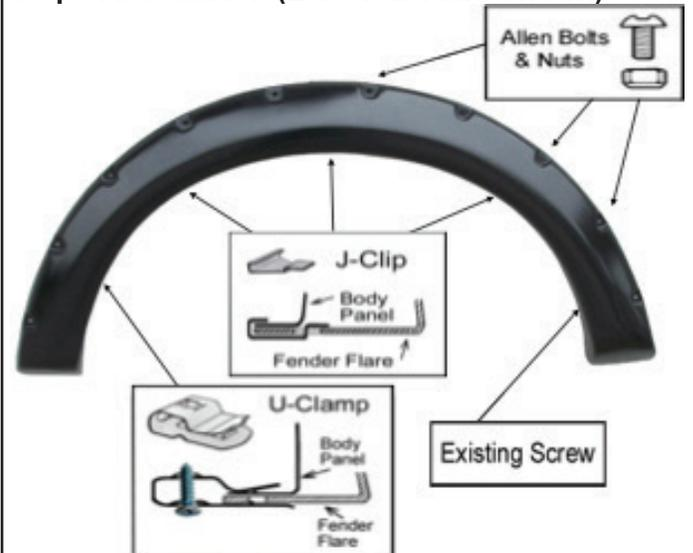
Use torx bit to tighten allen bolt & put firmly on every pocket of the fender flares. Place the flare on the vehicle. Apply 3 J-Clips into the mounting slots in the flare and secure it to the vehicle, 1 U-Clamp secure into the hole with flat head screw as shown. Fasten the existing factory screws into the original location that were preciously removed.
