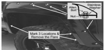
Use Torx Bit to tight allen bolt & nylon nut firmly on every pocket of the fender flares. **DO NOT OVER TIGHTEN!** Hold the flare firmly on the fender, to confirm the right position. Make sure other holes are on the position, use a grease pencil to mark 3 holes through the holes on the flare, as shown. Remove the flare.
