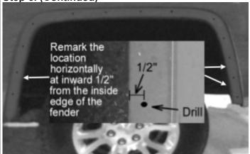
Remark the 3 locations horizontally at inward 1/2" from the inside edge of the fender. Drill a hole on the marked locations through sheet metal with a 3/32" drill bit. (Use a floor jack on the rear hitch to raise the truck bed for easy to drill.)
