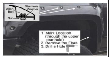
Use Torx Bit to tight allen bolt & nylon nut firmly on every pocket of the fender flares. **DO NOT OVER TIGHTEN!** Hold the flare firmly on the fender, to confirm the right position.
