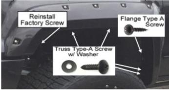
Install 4 supplied truss type A screws into the factory holes. Re-install the factory screw. Install 1 supplied flange type A screw into the hole drilled.
