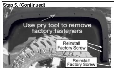
Pull the lower grip part to remove the factory flare from the vehicle. Use pry tool to remove any remaining factory fasteners.
