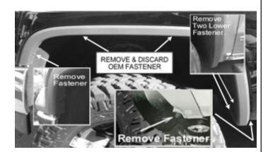
Use a 9/32" or 7mm socket to remove the fastener on the front of factory wheel arch molding (left shown). Use a T-15 Torx Bit to remove two lower fasteners on the rear of the factory wheel arch molding (right top shown). Use a 1/2" socket to remove fastener from the rear underside of factory wheel arch molding. Save and reinstallation. Use a T-15 Torx Bit to remove two fasteners along the top of the factory wheel arch molding (center top shown).
