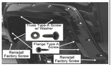
Install 3 supplied truss type A screws into the factory holes. Re-install the 2 factory screws underside. Install 3 supplied flage type A screws into the holes drilled.
