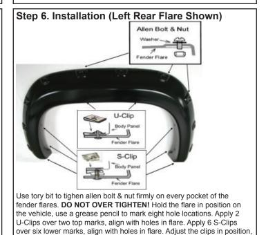
use 2 flange screws and 6 truss machine screws to secure it as shown.
