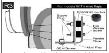
Insert the supplied spacer (10mm) in between vehicle body & flare, apply 2 hex washer screws on top two holes and 1 OEM screw on bottom hole, and secure the flare to the body.
