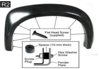
Fasten 7 flat heas screws into the location, shown as center. Insert the supplied spacer (10mm) in between vehicle body & flare, apply 1 hex washer screw to secure the flare to the body.
