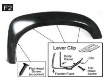
Apply 3 Lever Clip into the mountain slot in flare and secure it to the vehicle with flat head screw, shown as right. Fasten 1 flat head screw into the location, shown as left.
