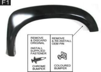
Remove fastener or pin from rear of bumper. Once the flares line up, attach and fasten it, shown as bottom.
