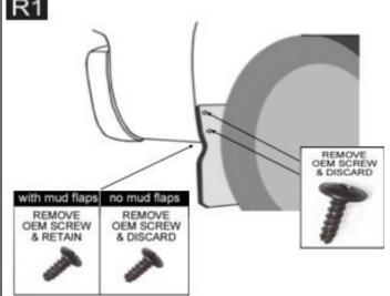
For the models with mud flaps, remove the 2 screws from the mud flap and discard, shown as right. Also remove the screws from the under side of the body and retain, shown as left.
