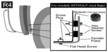
Insert the supplied spacer (10mm) in between vehicle body & flare, apply 2 hex washer screws on top two holes and 1 flat head screw on bottom hole, and secure the flare to the body.
