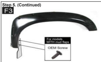
Re-Install the existing factory screws into the original location that were previously removed.
