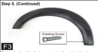
Fasten the 1 existing factory screw into the original location what was previously removed, as shown.
