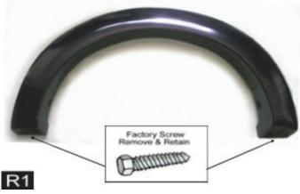
Remove the two existing factory screws with proper wrench and save it for reinstallation as shown.
