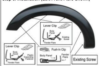
Place the flare on the vehicle. Apply 2 Push-In Clips into the mounting slot in the flare and secure it to the vehicle into the hole with existing screw & 3 Lever Clips secure plastic expanding fastener as shown. Fasten the existing factory screw into the original location that were previously removed.
