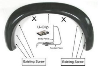
Remove 6 existing factory screws from the vehicle. Do not remove the two factory screws on the top center (marked with X). Apply 1 U-Clip over existing factory holes. Place the flare on the vehicle with best position. Fasten the existing factory screws into the original location that were previously removed. Press firmly on the flare, tighten all screws and secure it to the vehicle as shown.
