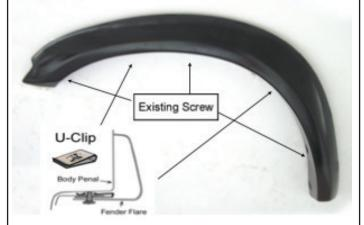
Remove 3 existing factory screws from the vehicle. Apply 2 U-Clips over the existing factory holes, on the top center use the one toward the front of the vehicle. Place the flare on the vehicle with best position. Fasten the existing factory screws into the original location that were previously removed. Press firmly on the flare, tighten all screws and secure it to the vehicle as shown.
