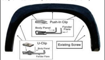
Place the flare on the vehicle. Apply 3 Push-In Clips into the mounting slots in the flare and secure it to the vehicle. Use 4 U-Clamps and secure into the hole with flat head screw as shown. Fasten the existing factory screws into the original location that were previously removed.
