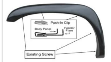
Place the flare on the vehicle. Apply 2 Push-In Clips into the mounting slot in the flare and secure it to the vehicle as shown. Fasten the existing factory scews into the original location that were previously removed.
