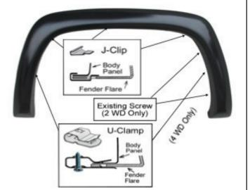
Place the flare on the vehicle. Apply 3 J-Clips into the mounting slots in the flare and secure it to the vehicle. Use 2 U-Clamps and secure into the hole with flat head screw as shown. Fasten the existing factory screws into the original location that were previously removed for 2 WD.
