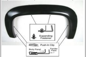
Place the flare on the vehicle. Apply 2 Plastic Expanding Fastener into the mounting slot in flare and secure it to the vehicle as shown. Apply 4 Push-In Clip into the mounting slot in the flare and secure itto the vehicle as shown.
