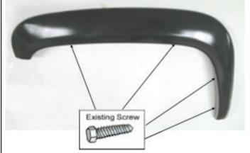
Remove 4 existing screws from the fasteners on the vehicle. Place the flare on the vehicle. Reinstall the existing factory screws into the original location that were previously removed. Do not tighten the screws fully until the flare are aligned and extrusive against the body.
