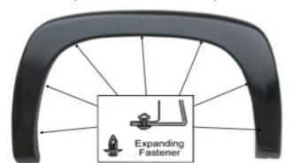
Place the flare on the vehicle. Apply 7 Plastic Expanding Fastender into the mounting slots in flare and secure it to the vehicle as shown.
