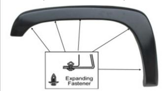
Place the flare on the vehicle. Apply 5 Plastic Expanding Fastener into the mounting slots in flare and secure it to the vehicle as shown.
