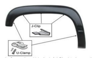
Place the flare on the vehicle. Apply 3 J-Clips into the mounting slots in the flare and secure it to the vehicle. Use 2 U-Clamps and secure it into the hole with hex screws as shown.
