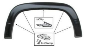
Place the flare on the vehicle. Apply 1 J-Clip into the mounting slots in the flare and secure it to the vehicle. Use 4 U-Clamps and secure it into the hole with hex screws as shown.
