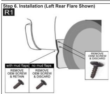
For the models with mud flaps, remove the 2 screws from the mud flap and discard, shown as right. Also remove the screws from the under side of the body and retain, shown as left.
