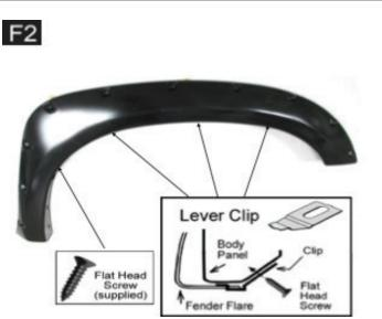
Apply 3 Lever Clips into the mounting slot in flare and secure it to the vehicle with flat head screw, shown as right. Fasten 1 flat head screw into the location, shown as left.
