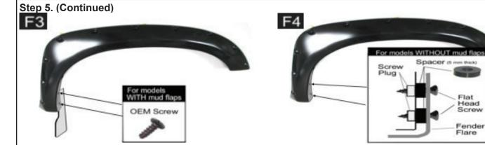
Re-Install the existing factory screws into the original location that were previously removed. Insert the apply 2 fla
