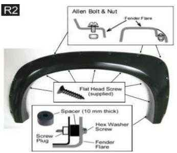
Use tory bit to tighten allen bolt & put firmly on every pocket of the fender flare, shown as top. Fasten 7 flat head screws into the location, shown as center. Insert the supplied spacer (10mm) in between vehicle body & flare, apply 1 hex washer screw to secure the flare to the body.
