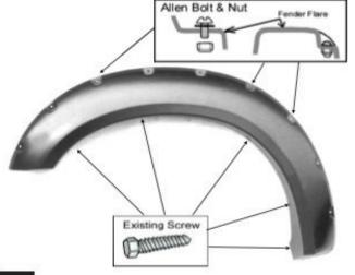
Use torx bit to tighten allen bolt & put firmly on every pocket of the fender flares. DO NOT OVER TIGHTEN! Remove 5 existing screws from the vehicle. Place the flare on the vehicle. Re-Install the existing factory screws into the original location that were previously removed. Do not tighten the screws fully until the flare are aligned and extrusive against the body.
