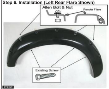
Use torx bit to tighten allen bolt & put firmly on every pocket of the fender flares. Place the flare on the vehicle. Apply 5 Push-In Clips into the mounting slot in the flares and secure it to the vehicle as shown.
