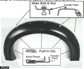
Use torx bit to tighten allen bolt & put firmly on every pocket of the fender flares. Place the flare on the vehicle. Fasten the existing factory screws into the original location that were previously removed.
