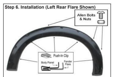
Use torx bit to tighten allen bolt & put firmly on every pocket of the fender flares. Place the flare on the vehicle. Apply 5 Push-In Clips into the mounting slot in flare and secure it to the vehicle as shown.
