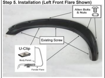
Use torx bit to tighten allen bolt & put firmly on every pocket of the fender flares first. DO NOT OVER TIGHTEN! Remove 3 existing factory screws from the vehicle. Apply 2 U-Clips over existing factory holes, on the top center, use the one towards the front of the vehicle. Place the flare on the vehicle. Fasten the existing factory screws into the original location that were previously removed. Press firmly on the flare, and tighten all screws and secure it to the vehicle as shown.
