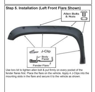
Qty (4) U-Clamp with Flat Head Screw Qty (14) J-Clip Qty (36) Allen Bolt & Nut (Torx Bit required) Qty (8) Self Tapping Screws (see **option B**)
