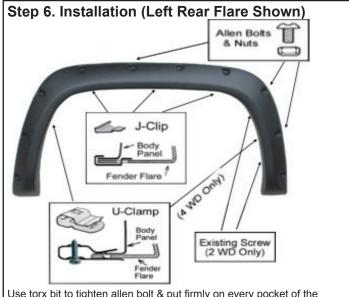
Use torx bit to tighten allen bolt & put firmly on every pocket of the fender flares first. Place the flare on the vehicle. Apply 3 J-Clip into the mounting slots in the flare and secure it to the vehicle. Use 2 U-Clamps and secure it into the hole with flat head screws as shown. Fasten the existing factory screws into the original location what were previously removed for 2 WD.
