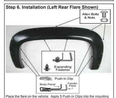
slots in the flare and secure it to the vehicle as shown.
