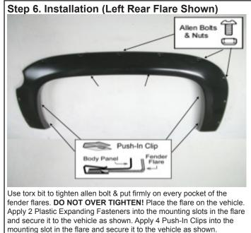
Option B: If condition of fender prevents use of the push-in clips you can use the included self tapping screws to secure the flare to the fender.
