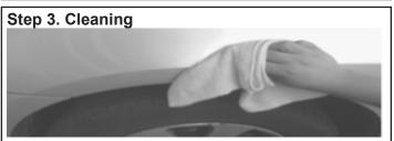
Wash and wipe dry the areas of contact on the vehicle body. Clean the surface and inside edge of the fender flare where the rubber seal is to be attached.
