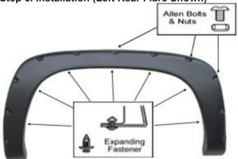
Use torx bit to tighten allen bolt & put firmly on every pocket of the fender flares first. Place the flare on the vehicle. Apply 7 Plastic Expanding Fasteners into the mounting slots in the flare and secure it to the vehicle as shown.
