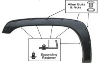
Use torx bit to tighten allen bolt & put firmly on every pocket of the fender flares first. Place the flare on the vehicle. Apply 5 Plastic Expanding Fasteners into the mounting slots in the flare and secure it to the vehicle as shown.
