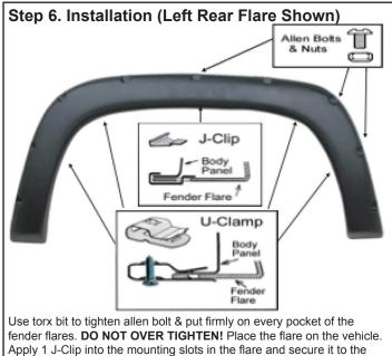
vehicle. Use 4 U-Clamps and secure it into the hole with hex screws as
