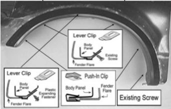
Place the flare on the vehicle. Apply 3 Lever Clips, secure it to the hole with existing screws as shown. Fasten the existing factory 2 screws into the original location that were previously removed.
