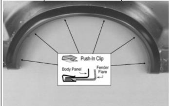
Place the flare on the vehicle. Apply 3 J-Clips into the mounting slots in the flare and secure it to the vehicle, 1 U-Clamp secures into the hole with flat head screws as shown. Fasten the existing 3 factory screws into the original location that were previously removed.
