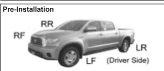
Prefit both driver side and passenger side fender flares to the vehicle before painting or installation. You may remove any moldings, strips or existing flares from the vehicle for fitting or installation. You can cut the fender flare to fit any body side molding.
