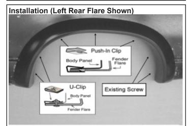
Place the flare on the vehicle. Apply 3 Push-In Clips into the mounting slots in the flare and secure it to the vehicle, 4 U-Clips secure into the hole with screws as shown. Fasten the existing factory screws into the original location that were previously removed.
