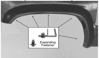
Place the flare on the vehicle. Apply 5 Plastic Expanding Fastener into the mounting slots in flare and secure it to the vehicle as shown.
