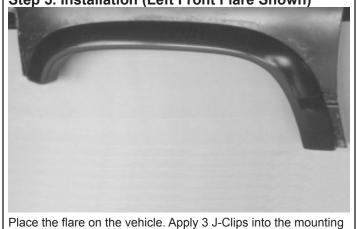
slots in the flare and secure it to the vehicle. Use 2 U-Clamps
